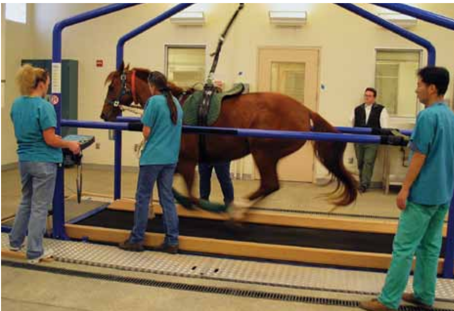
The Claire Giannini Equine Athletic Performance Laboratory features both research and clinical diagnostic treadmills to evaluate horses under exercise conditions.
