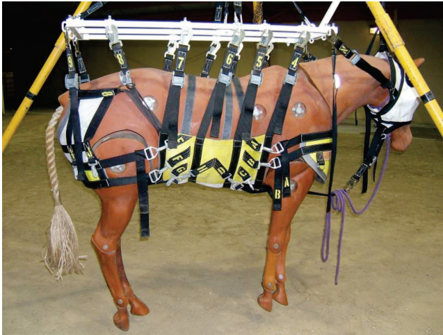
Fig. 1. Lucky, the training dummy, hangs in the UCD Anderson Sling. Notice that the load is distributed throughout the abdomen and thorax as well as the rump and pectoral region.
