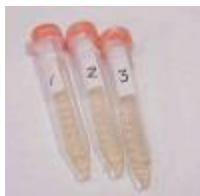
These three screw-cap tubes contain specimens being sent to a laboratory for diagnostic testing. The tubes have been sealed with parafilm, to prevent leakage around the cap. Parafilm should always be on hand when you package your samples for shipping.
