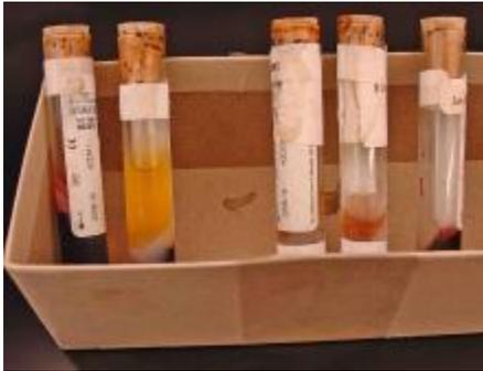
Tubes with cork stoppers are NOT acceptable; evidence of leakage is visible on the labels and in the box.
