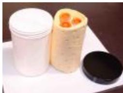
Tubes should be packed with absorbent material into a leak-proof secondary container. Multiple primary receptacles are individually wrapped to prevent contact between them. The absorbent material must be sufficient to absorb the entire contents of the primary containers.
