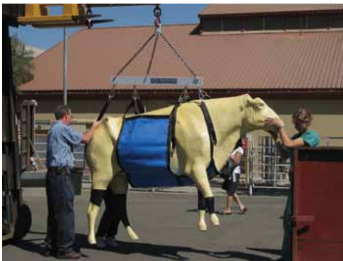
Using a life-sized bovine model, Professor John Madigan and Dana Conly, class of 2009, demonstrate a specialized sling system developed at the school's teaching hospital. The sling is used to safely lift a recumbent animal into a therapeutic flotation tank for support while recovering from a fall, a difficult birth on a dairy, or other medical condition.
