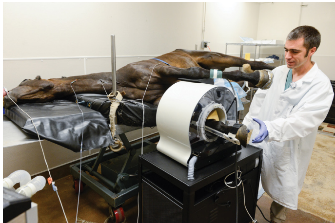
Dr. Mathieu Spriet positions a horse's leg in UC Davis' new portable PET scanner.
