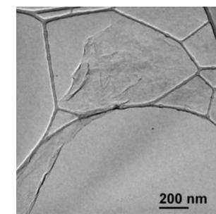
Fig. 4: Transmission Electron Microscopy (TEM) image of GO (250nm x 250nm).
