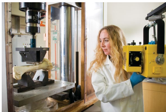
The Materials Testing System tests the mechanical strength of an equine bone in the J.D. Wheat Veterinary Orthopedic Research Laboratory.
