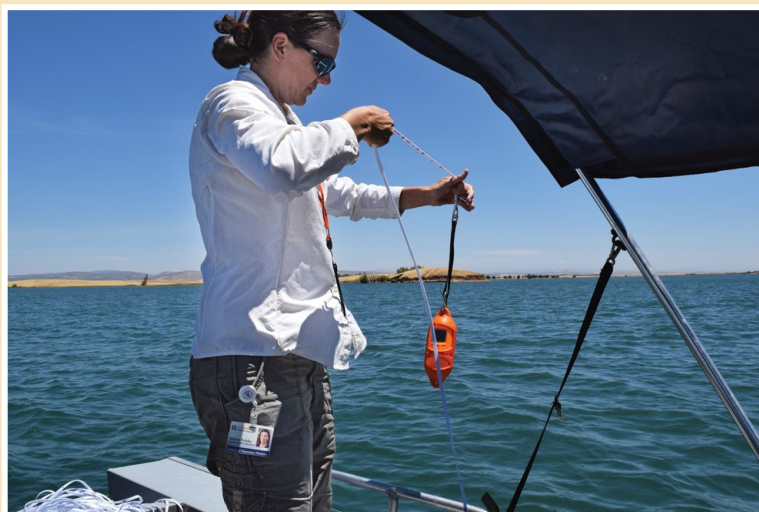
Melissa Partyka retrieves a conductivity, temperature, depth (CTD) profiler from a Central Valley reservoir.
